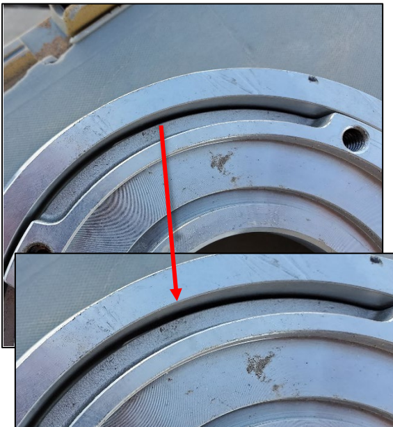
Obvious gap between adjusting ring and base
